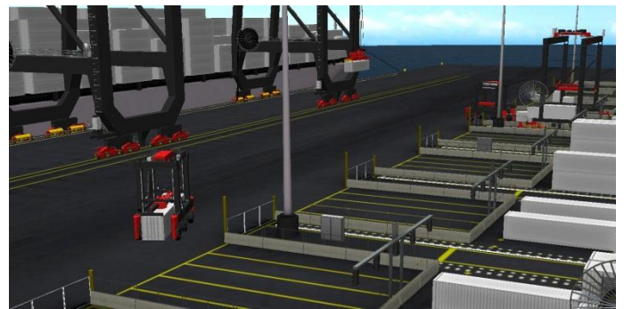
Waterside horizontal transport with shuttle carriers in the end-loading ASC layout
