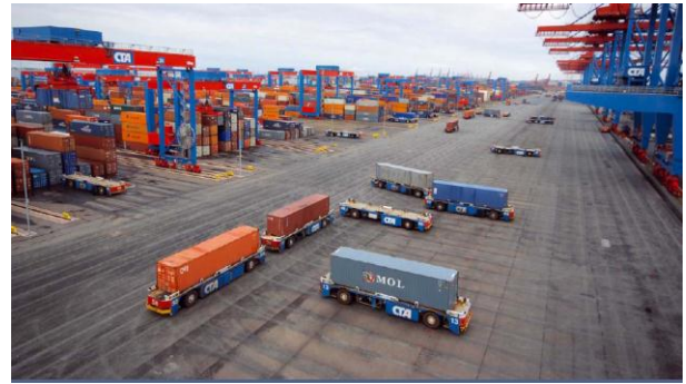
AGVs at Container Terminal Altenwerder, Hamburg
