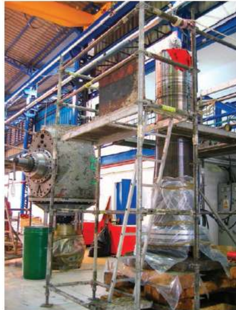
Azimuth thrusters being disassembled at the Multipurpose Work
