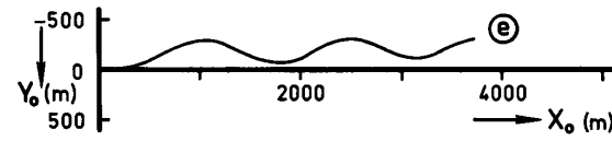
Figure 54 Time Histories and x-y Plot of Zig-zag Test L (30/20) at 60 Nominal RPM
