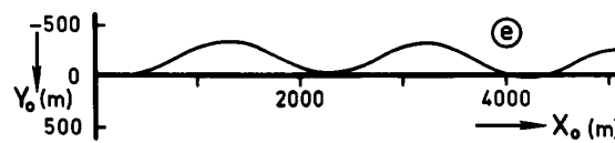
Figure 53 Time Histories and x-y Plot of Zig-Zag Test J (20/20) at 70 Nominal RPM
