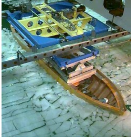
Figure 4.3: Model test with PMM in ice performed by Oceanic Consulting Corporation [1]
