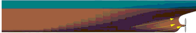
Figure 7.7: Upward oblique flow in the ship stern area (side view)
