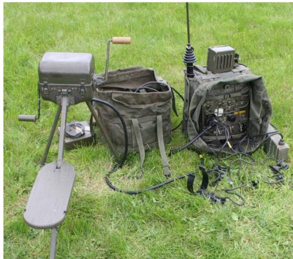
**Figura 10 - E/R de HF, AN/GRC-9, pronto a operar**
