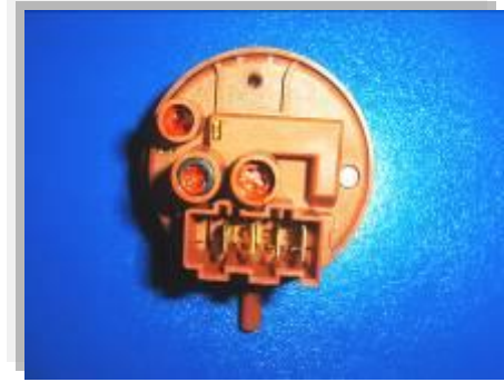
Figure 9. Pressure switch
