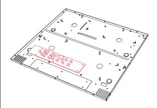
Step 7: remove the display board
