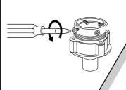
Connect the water tap adapter to the water tap tighten the four screws evenly while pushing up the adapter so that the rubber packing can stick to the water tap tightly.
