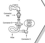
3 Insert the inlet hose adapter into the water inlet of a washer and turn it to be fixed.
