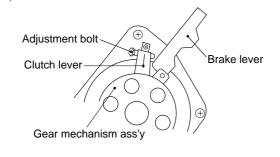
i Tighten the link brake screw completely.
