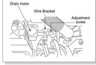
Separate the drain motor from the bracket.
