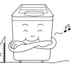
Keep the machine body more than 25cm apart from the wall surface. It will make easy cleaning the drain filter which is equipped at the back side of it. And if it comes into contract vibration may occur.
