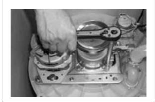
¡ Pull out the gear mechanism assy.
