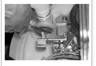
i Remove the valve lid from the valve drain assy.
