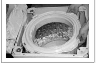
Loosen the pulsator mounting screw and remove the pulsator.
