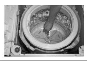
; Remove the spinner shaft flange nut by using 'T' type box wrench.
