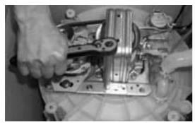
; Remove four bolts mounting the gear mechanism ass'y by using a box wrench.
