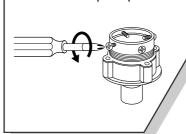
Connect the water tap 3 adapter to the water tap tighten the four screws evenly while pushing up the adapter so that the rubber packing can stick to the water tap tightly.
