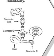
3 Insert the inlet hose adapter into the water inlet of a washer and turn it to be fixed.
