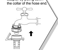
Connect the inlet hose adapter Of the hose to the water inlet of the washer by turning it clockwise to be fixed tightly.
