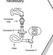
Insert the inier riose data. Insert the inlet hose adapter and turn it to be fixed.
