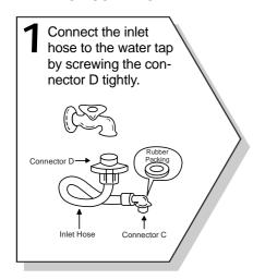
Connect the connector-inlet supplied if necessary.
