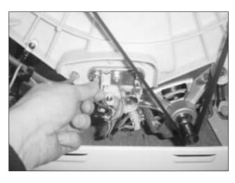
3) Remove the nut by using a box wrench, and remove the earth terminal.
