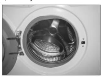
4) Remove two screws, and push the door lock switch to the right direction.
