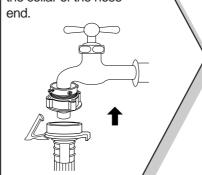
6 Connect the inlet hose adapter of the hose to the water inlet of the washer by turning it clockwise to be fixed tightly.
