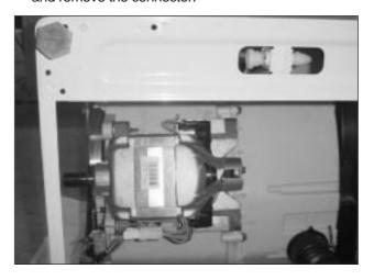
4) Remove the motor from the tub.
