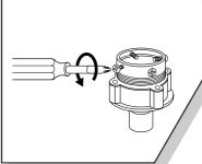
(3) Fit the water tap adapter into the water tap and tighten the four screws evenly while pushing up the adapter so that
