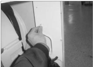
3) Remove the screw, and remove the drain pump from
