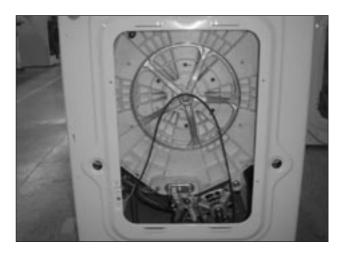
3) Remove two bolts and two nuts mounting the motor by using a box wrench.
