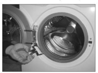
3) Remove two screws, and remove the door lock
