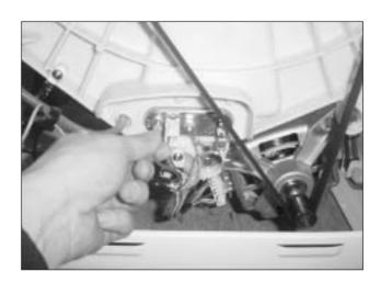
3) Remove the nut by using a box wrench, and remove the earth terminal.
