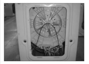
3) Remove two bolts mounting the motor by using a box wrench.
