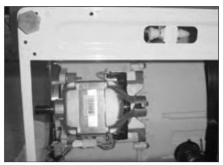
4) Remove the motor from the tub.
