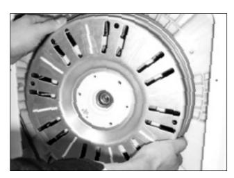
4) Separate the STATOR from the TUB.
