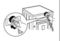
• Check the packing in the inlet.
