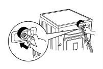
• Check the packing in the inlet.
