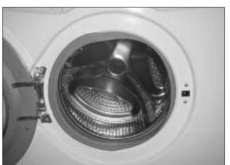
3) Remove two screws, and remove the door lock switch.
