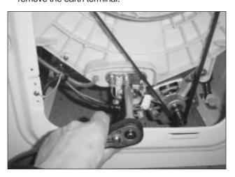
4) Loosen the nut by using a box wrench, and pull out the heater.
