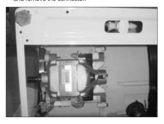
4) Remove the motor from the tub.
