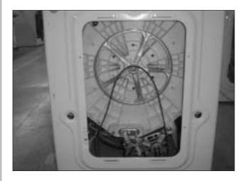
3) Remove two bolts mounting the motor by using a box wrench.
