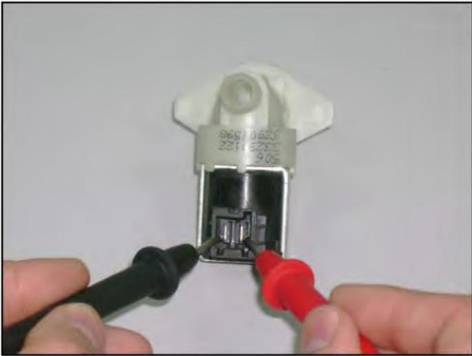
Probes of the tester should be applied on to the related connectors as shown on the pictures.
