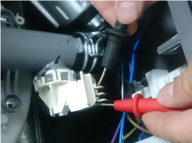
Probes of the tester should be applied on to the related connectors as shown in the picture above.
