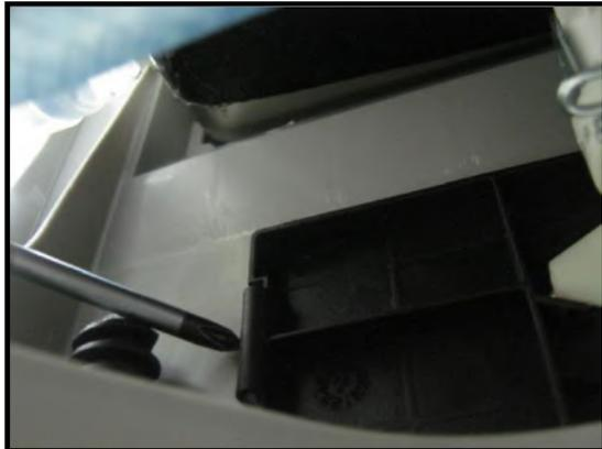
b) By using flat tip screwdriver remove hose connection plastic's hinge from the basement as it shown in the picture
