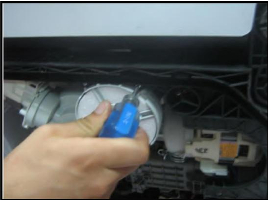
b) Remove two screws that fix floater as it is shown in the picture.
