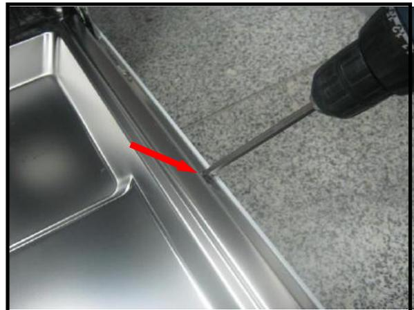
b) Pull down the front panel after removing the screws.
