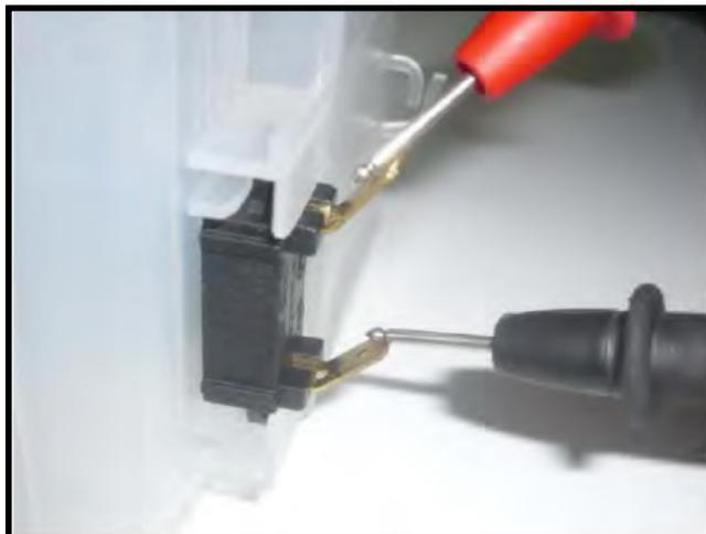
salt sensor can also be measured from the water softener when the salt sensor is assembled on the water softener.
