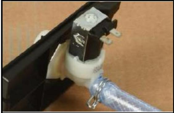
Above sketch show the connectors of the water inlet valve on the electrical card. Probes of the tester should be applies on to the related connectors.
