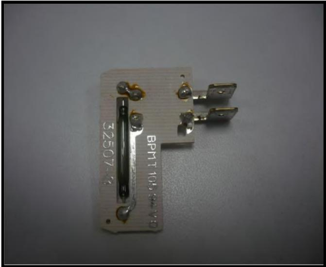
Above sketch shows the connectors of the rinse aid sensor on the electrical card.
