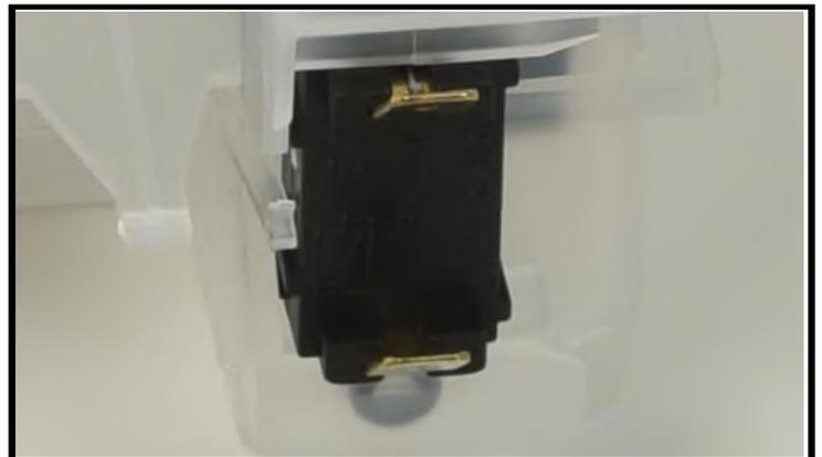
Sketch above show the connectors of the salt sensor on the electrical card. Probes of the tester should be applied on the related connectors.
