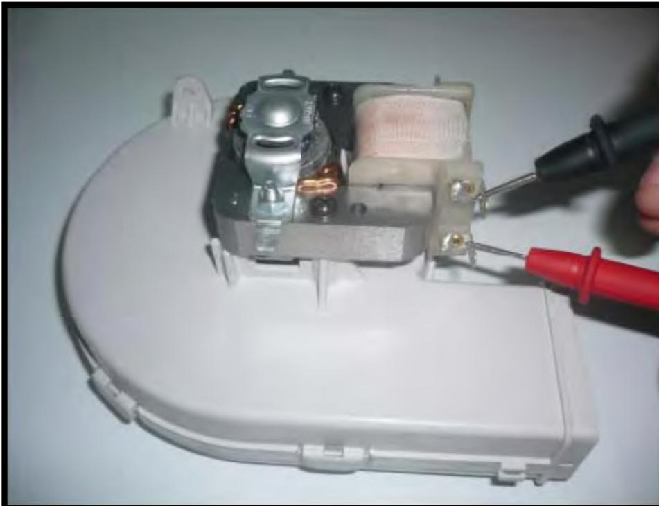
Probes of the tester should be applied on to the related connectors as shown on the pictures.
