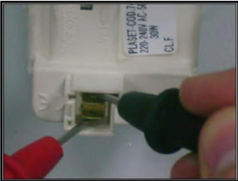
Probes of the tester should be applied on the related connectors as shown on the pictures.
