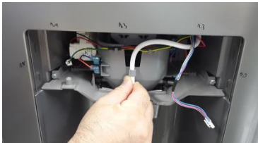
Separate a Water Hose which is assembled at dispenser guide
