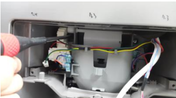
Loosen 4 screws for fixing a dispenser guide.
