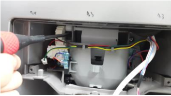
Loosen 4 screws for fixing a dispenser guide.
