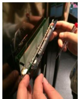
6/ Disconnect the terminal and replace a new interface set
