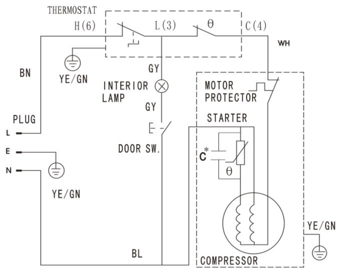
C\*: The capacitor is optional according to different compressor model
