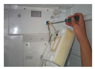
6) After romoving the control switch knob and two screws for fixing control switch, change the control switch to new one.
