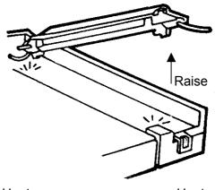
5) Pull out the glass tube heater from the heate supporter with heater covers remaining.(upper and lower) (Do not apply much power on the heater supporter.)
