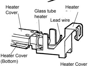
6) Install the heater covers (upper and lower) on a new glass tube heater. (Make the cover with holes the lower one)
