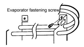
2) Slightly pull the evaporator to the arrow's direction.
