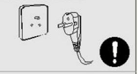
In case of damaged power cable When the power cable or plug has been worn, it is prohibited to continue to use it. In this case, it is required to replace it by factory authorized service shop
