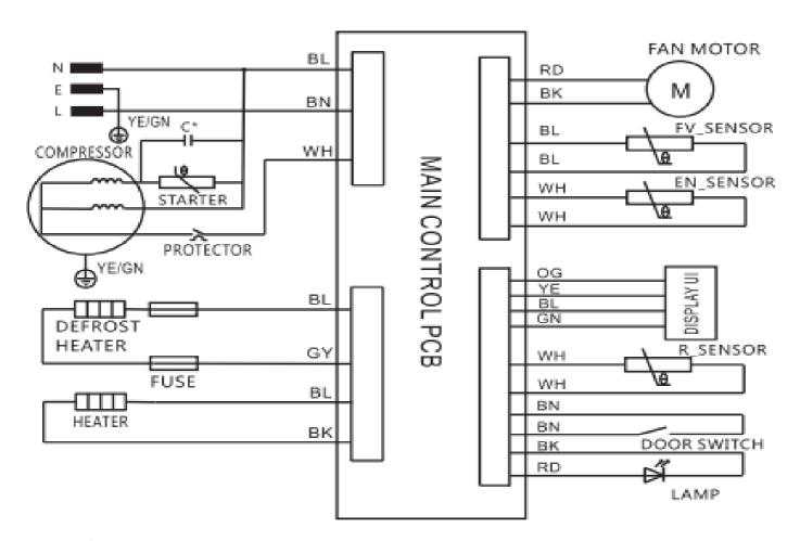
C\*: The capacitor is optional according to different compressor model
