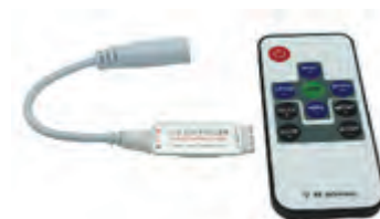
CT-RF-72W-RGB-MINI Dimensões: 35 x 15 x 4.5mm Input: 12VDC Output power < 72W Output current < 2A / Canal RF 433 MHZ WIRELESS SIGNAL CONTROL
