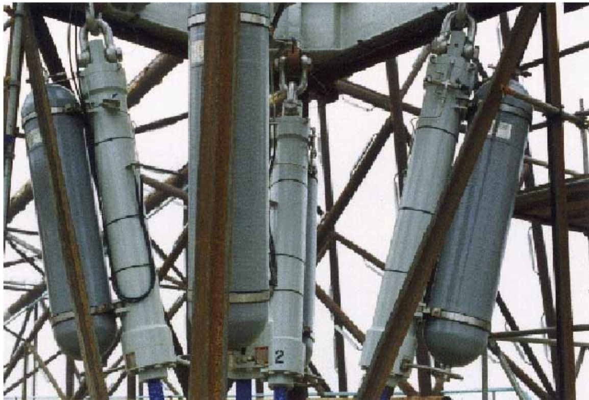
Figure 12. Riser tensioning assembly on a tension leg platform, showing composite high pressure gas accumulator bottles (Lincoln Composites).
