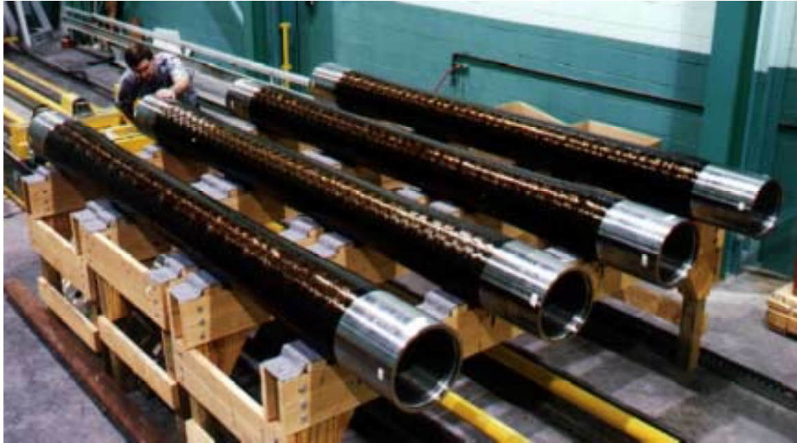
Figure 11. Composite production riser specimens prepared for qualification testing (Lincoln Composites).
