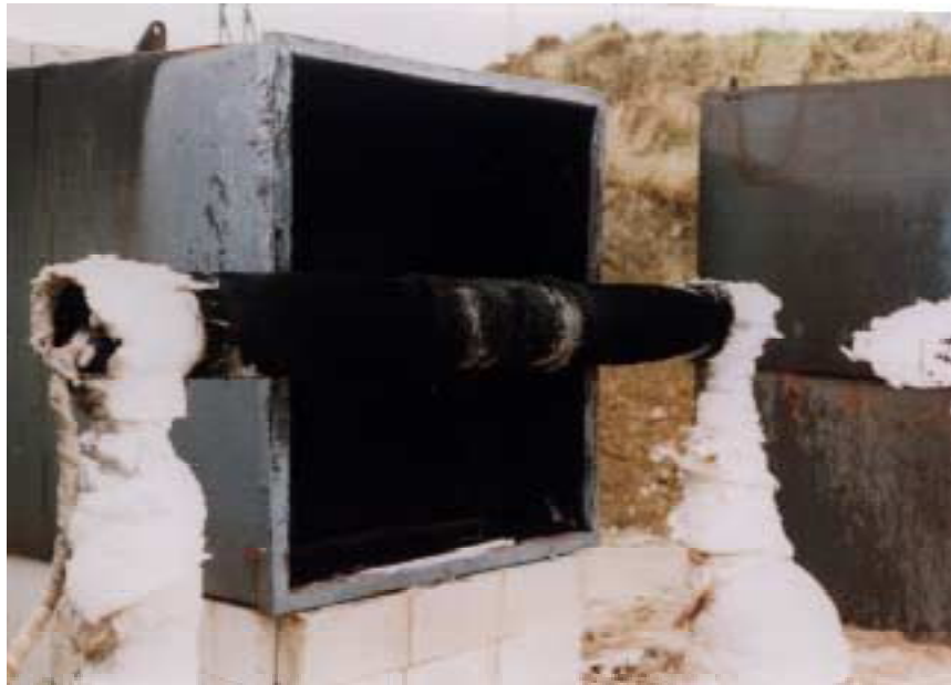
Figure 29. Jet fire test on a steel tubular with composite fire protection (upper photograph). Lower photograph shows specimen, with remaining protection and carbonaceous char after 2 hours in the test (Courtesy of Vosper Thornycroft and HSL Buxton).
