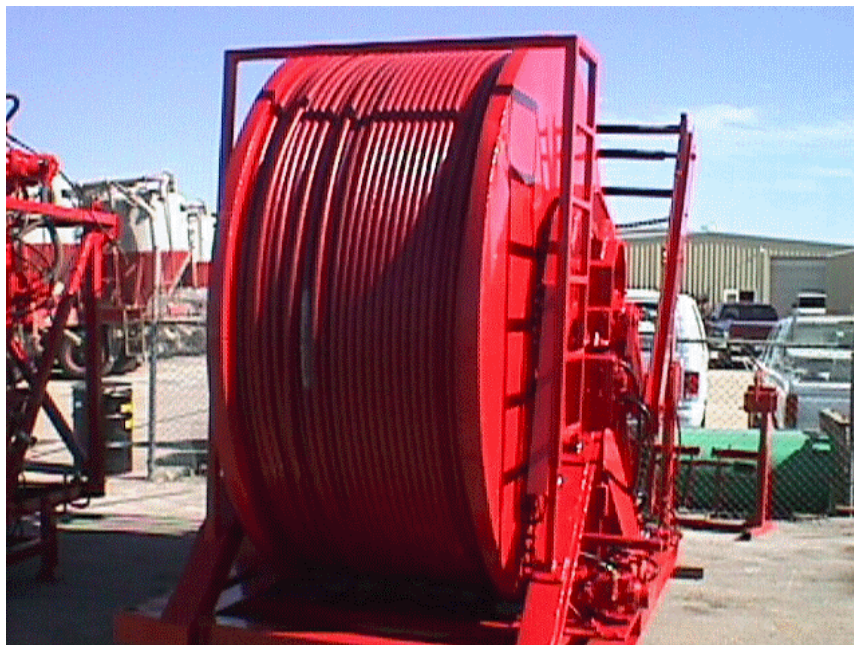
Figure 8. Flexible thermosetting composite tube (Courtesy of Fiberspar)
