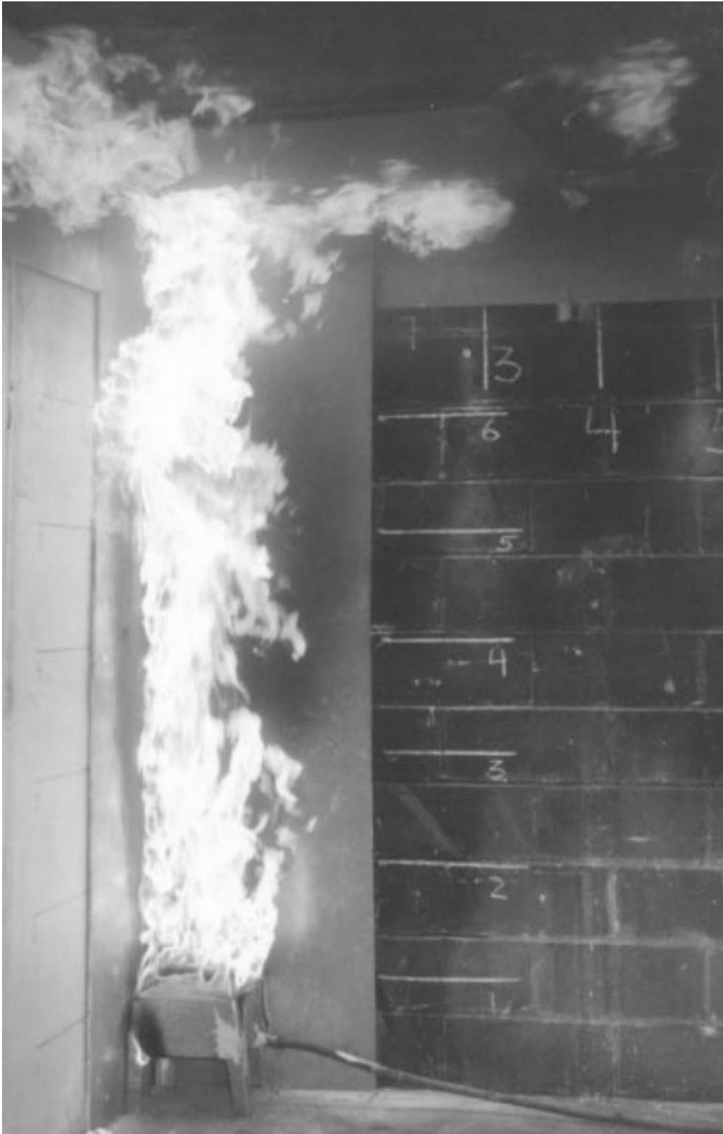
Figure 6-31 ISO 9705-Type Test with Reduced Material Quantities at VTEC Laboratories
