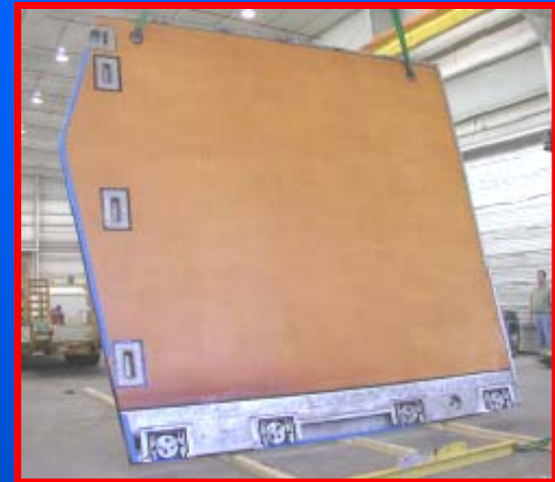
Composite Helicopter Hanger First Article Door (above) and Operational Test Jig (below) [Seemann Composites]
