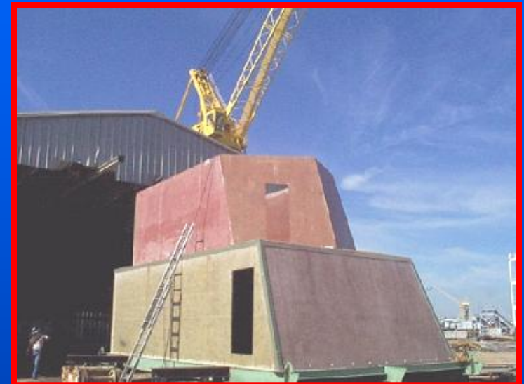
MARITECH Composite Superstructure Project Built by Structural Composites and Ingalls using Adhesive Technology
