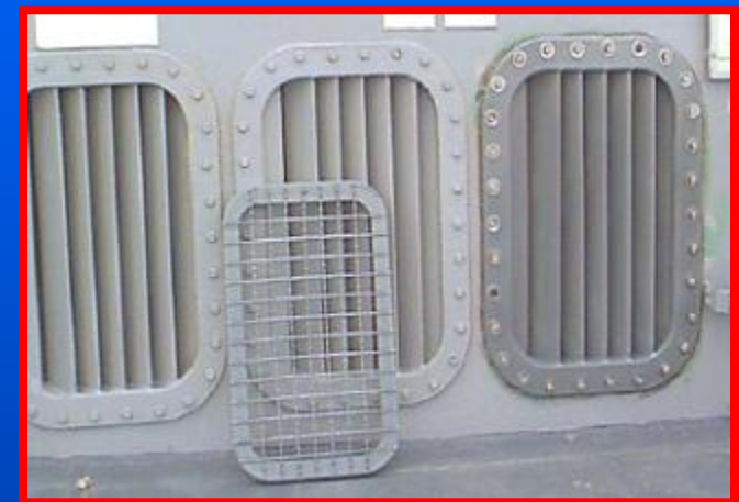
Radar Absorbing Composite Louver Developed for the DDG 51 Class Destroyers
