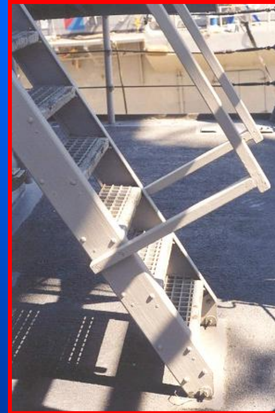
Composite Ladder Located Topside on FFG-58, the USS Samuel B. Roberts
