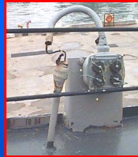
Typical Corrosion-Related Failure (above) and ULTEM 2300 Box Molded by Glenair (below)
