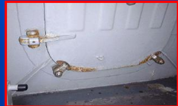
Watertight Door Showing Wear Due to Hinge Misalignment (above) and Corrosion (below)
