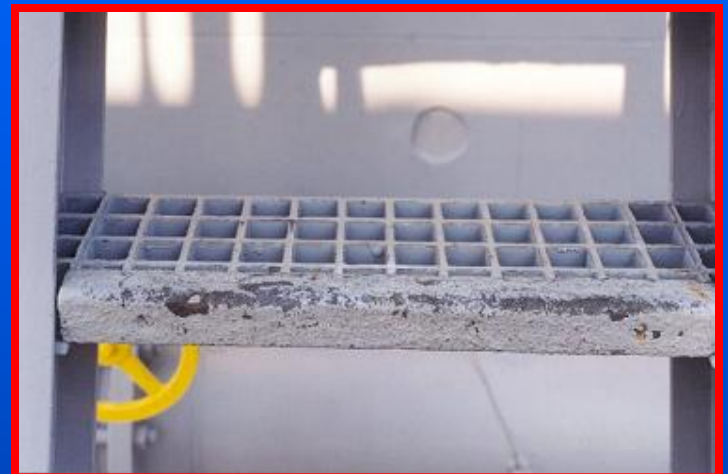
Topside Example of Stair Treads on the USS Samuel B. Roberts Showing Wear of Painted Finish
