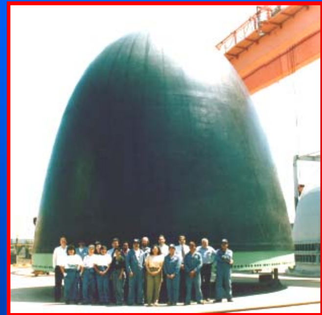
Composite Submarine Bow Dome Produced by Goodrich Composites
