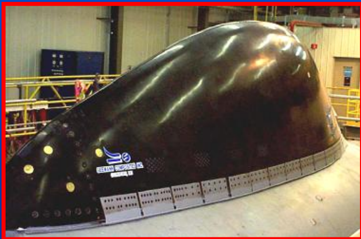
Advanced Composite Sail Envisioned for Virginia Class Submarines (top left) and 1/4-Scale Prototype Built by Seemann Composites (bottom left)
