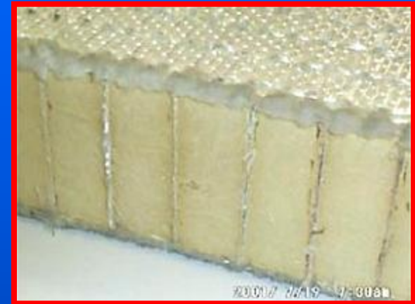
Webcore Hybrid Fabric- Web/Strut-Web Core with Pre-Attached Fabric Proposed for Navy SBIR Door Project
