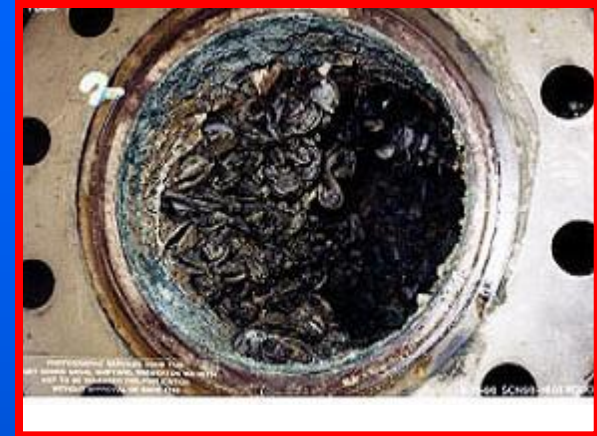
Example of Fouled Heat Exchanger Head Inlet (above) [ERM, Fred Tsao, 05L] and Relative Effectiveness of Composites (below) [Joseph Korczynski, NSWCCD]
