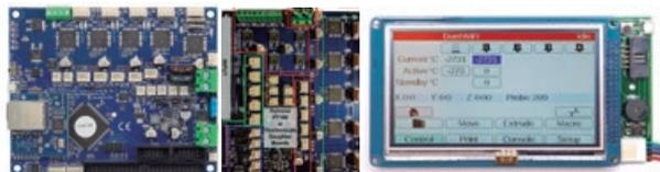
Figura 10. Placa Duet 2 Ethernet, Duex5 e PanelDue [16].
