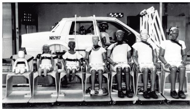
Figura 1. *General Motors crash test dummies: Hybrid II Series (1972).*
