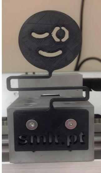
**Figure 2.** Acceleration test elastic element.
