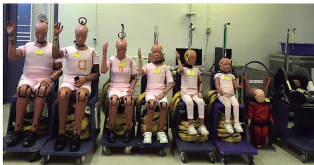
**Figura 2.** General Motors crash test dummies: Hybrid III Series (1997).
