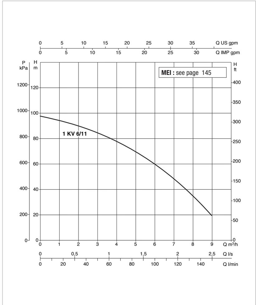
The performance curves are based on kinematic viscosity values = 1 mm²/s and density equal to 1000 kg/m³.
