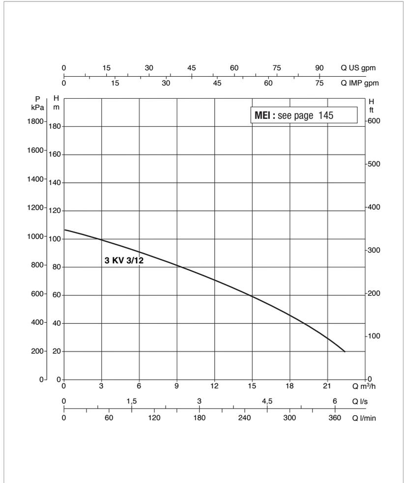
The performance curves are based on kinematic viscosity values = 1 mm²/s and density equal to 1000 kg/m³. Curve tolerance according to ISO 9906. **Overall performance taking into account THREE pumps working at the same time.** The performance results of sets with smaller pumps are obtained through simple calibration of the Active Driver module.
