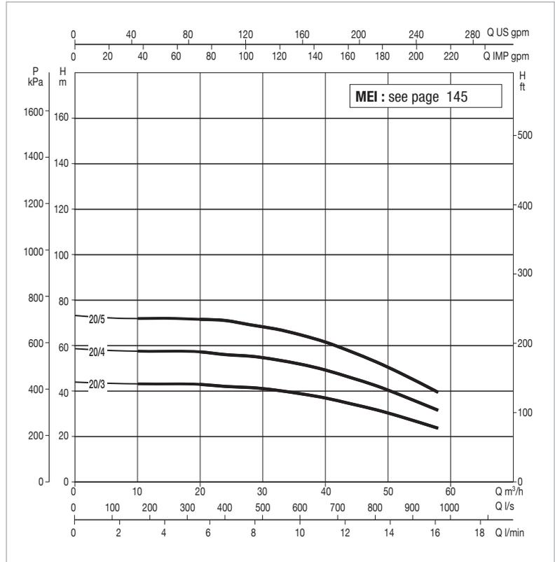
The performance curves are based on kinematic viscosity values = 1 mm<sup>2</sup>/s and density equal to 1000 kg/m<sup>3</sup>. Curve tolerance according to ISO 9906.
