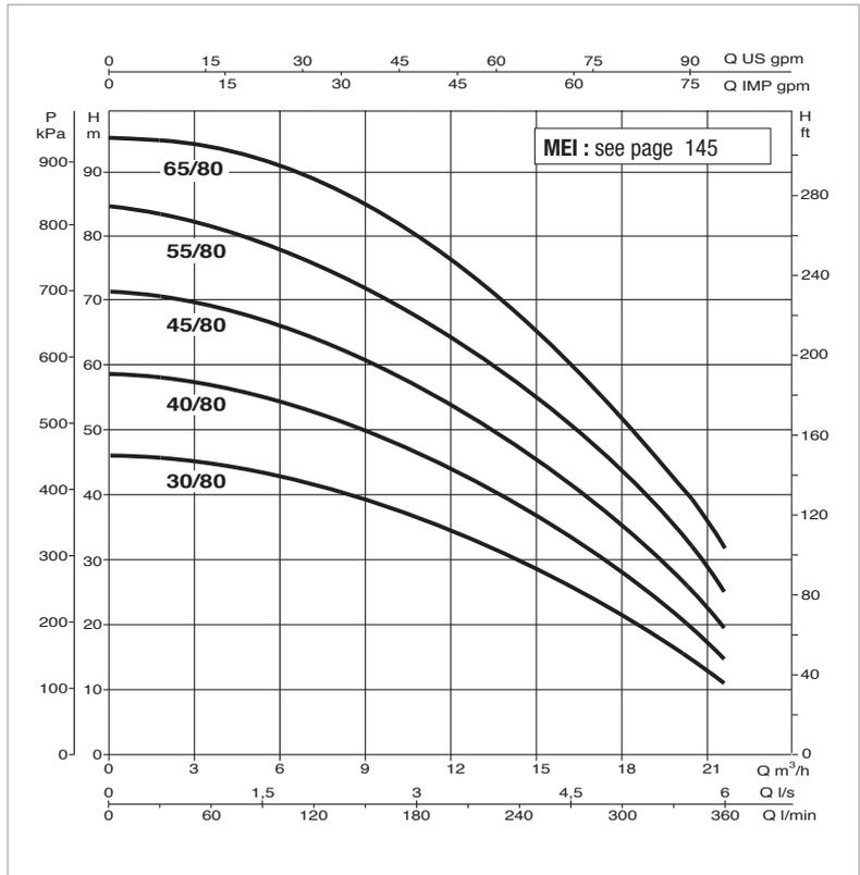
The performance curves are based on kinematic viscosity values = 1 mm<sup>2</sup>/s and density equivalent to 1000 kg/m<sup>3</sup>
