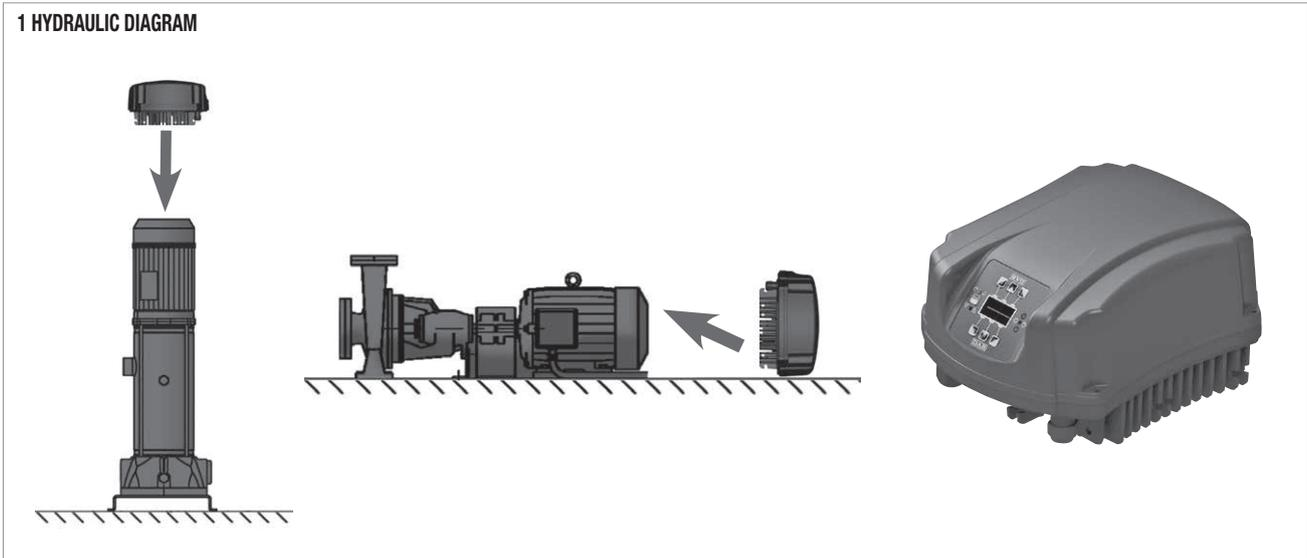
The MCE must be installed on the bottom of the motor.
