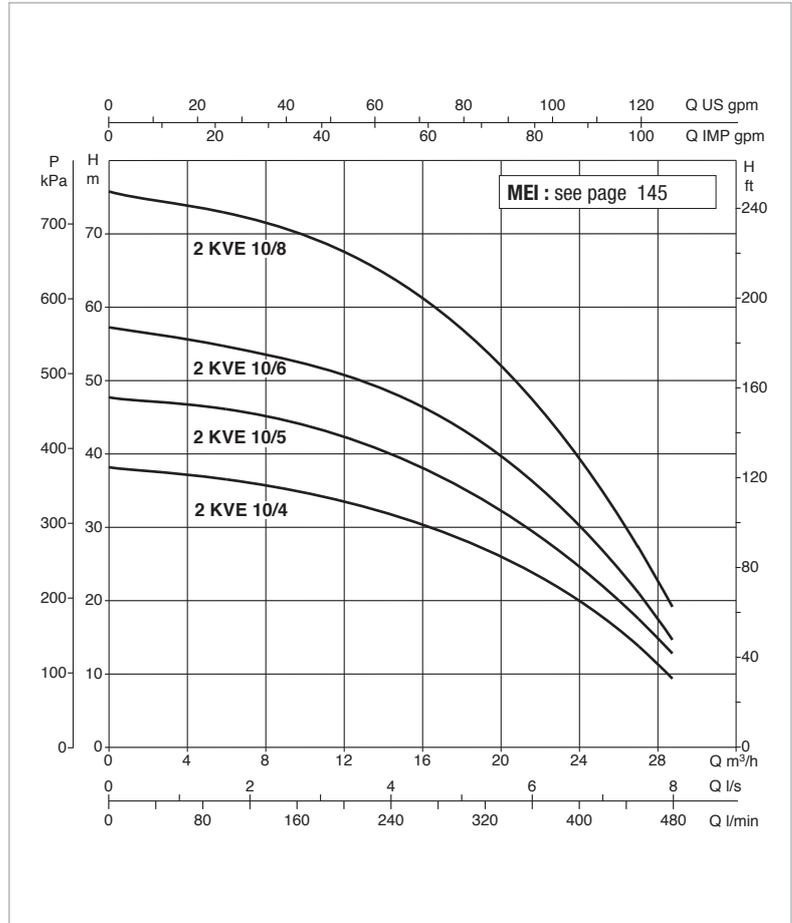
The performance curves are based on kinematic viscosity values = 1 mm<sup>2</sup>/s and density equal to 1000 kg/m<sup>3</sup>.
