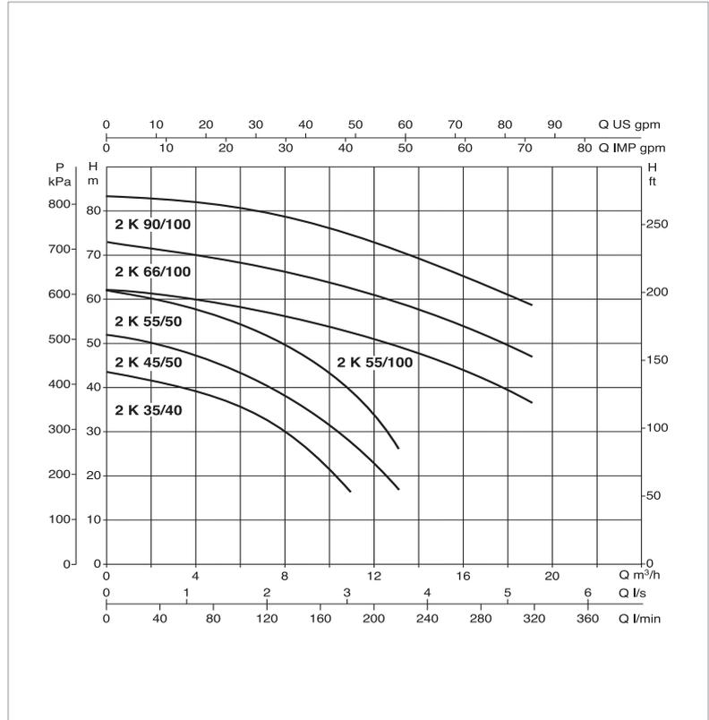
The performance curves are based on kinematic viscosity values = 1 mm²/s and density equivalent to 1000 kg/m³
