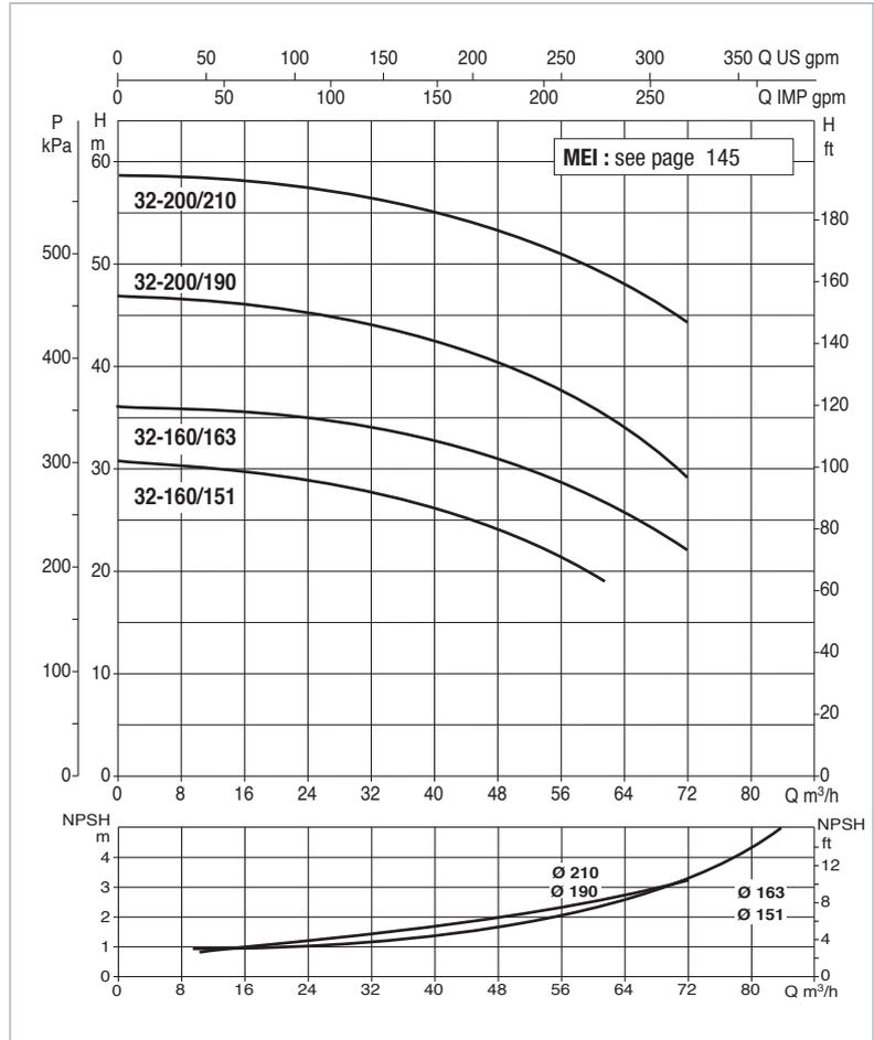
The performance curves are based on kinematic viscosity values = 1 mm<sup>2</sup>/s and density equivalent to 1000 kg/m<sup>3</sup>
