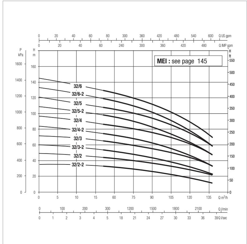
The performance curves are based on kinematic viscosity values = 1 mm<sup>2</sup>/s and density equal to 1000 kg/m<sup>3</sup>.
