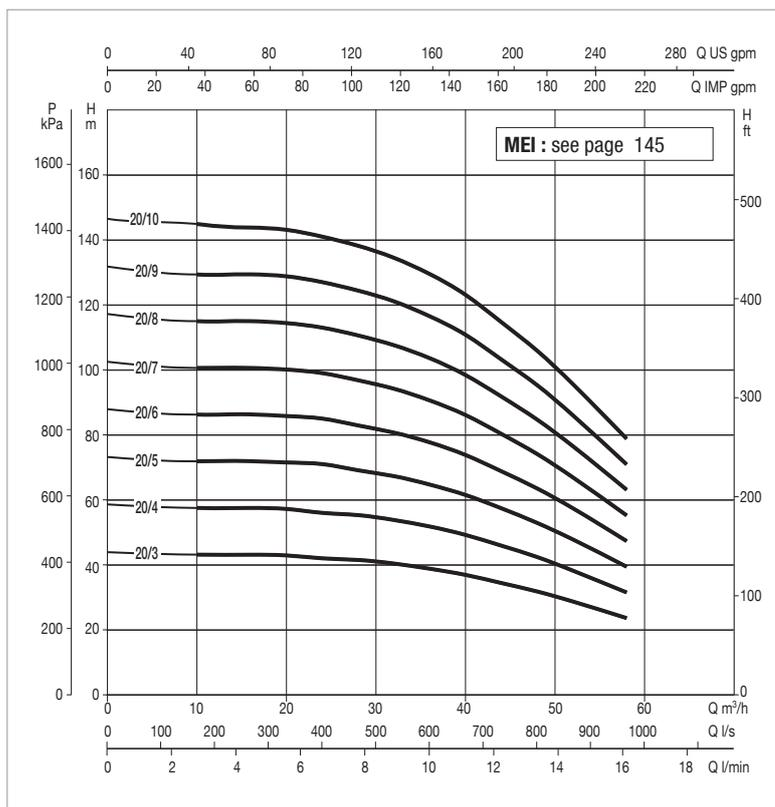
The performance curves are based on kinematic viscosity values = 1 mm<sup>2</sup>/s and density equal to 1000 kg/m<sup>3</sup>.
