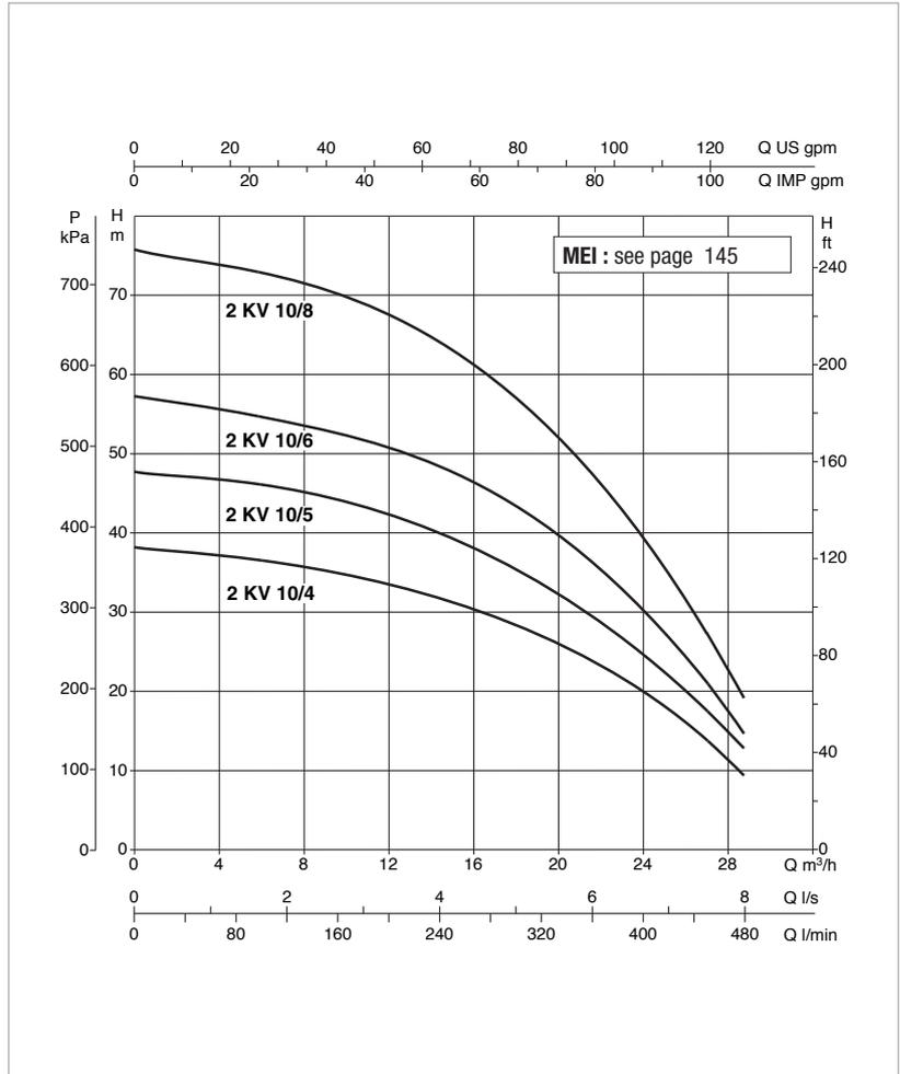
The performance curves are based on kinematic viscosity values = 1 mm<sup>2</sup>/s and density equal to 1000 kg/m<sup>3</sup>. Curve tolerance according to ISO 9906. **Overall performance taking into account TWO pumps working at the same time.** The performance results of sets with smaller pumps are obtained through simple calibration of the Active Driver module.
