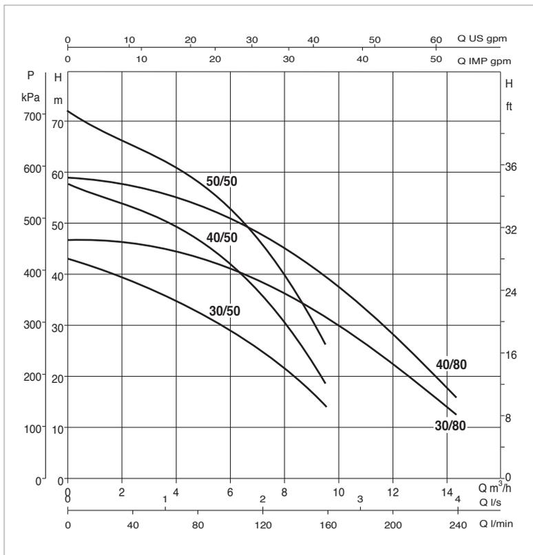
The performance curves are based on kinematic viscosity values = 1 mm<sup>2</sup>/s and density equivalent to 1000 kg/m<sup>3</sup>
