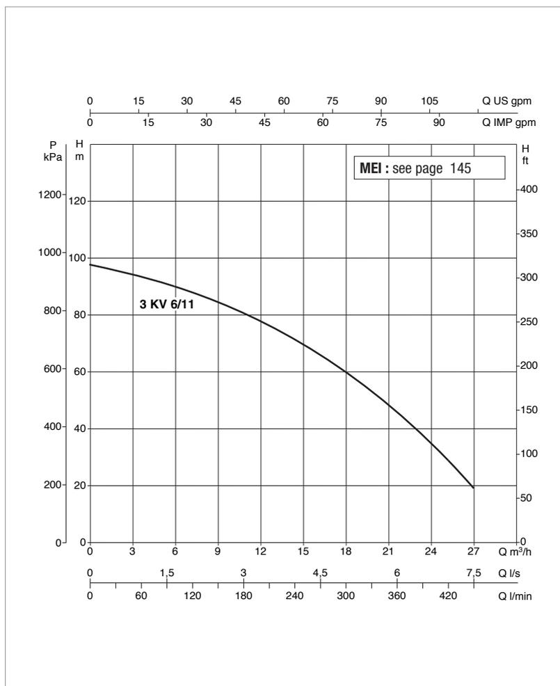
The performance curves are based on kinematic viscosity values = 1 mm<sup>2</sup>/s and density equal to 1000 kg/m<sup>3</sup>. Curve tolerance according to ISO 9906. **Overall performance taking into account THREE pumps working at the same time.** The performance results of sets with smaller pumps are obtained through simple calibration of the Active Driver module.
