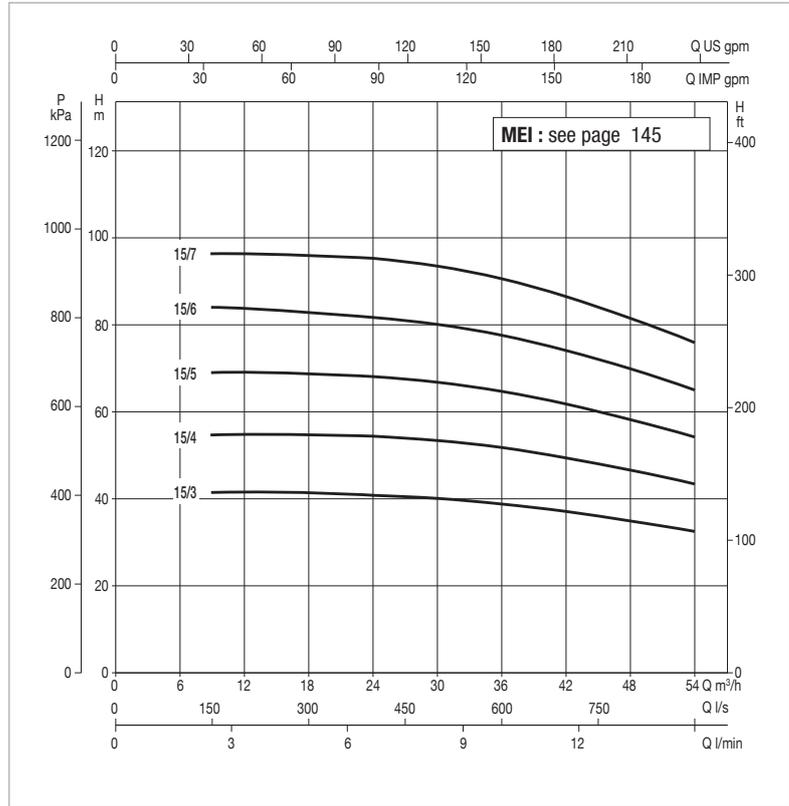
The performance curves are based on kinematic viscosity values = 1 mm²/s and density equal to 1000 kg/m³.
