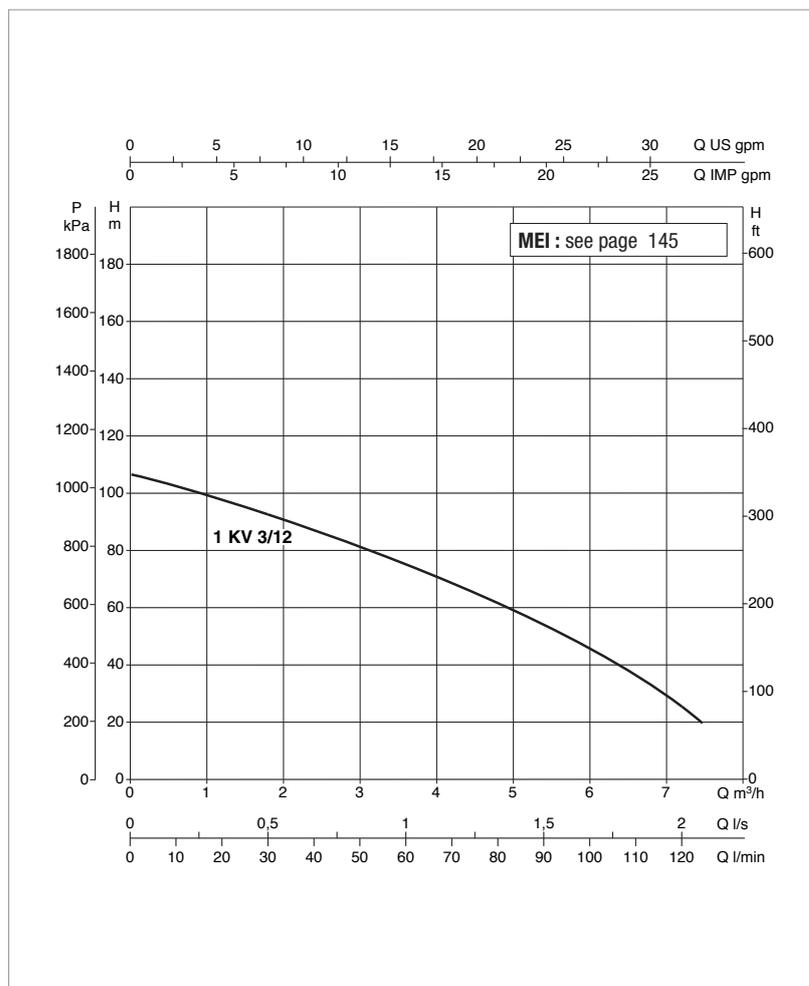
The performance curves are based on kinematic viscosity values = 1 mm<sup>2</sup>/s and density equal to 1000 kg/m<sup>3</sup>.
