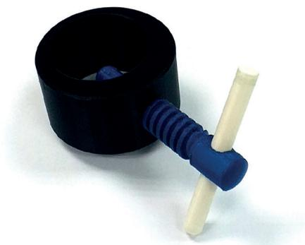
Figure 9. Final assembly of the nutcracker.
