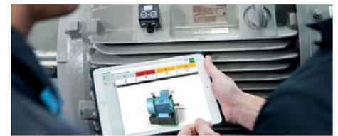
Figura 5. Schaeffler ConditionAnalyzer. M
