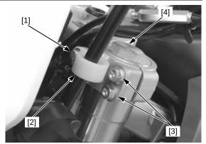
Loosen the fork bottom pinch bolts [1] while supporting the fork leg.
