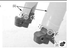
Install the brake hose clamp [1] to the left fork leg and tighten the bolts [2] to the specified torque.
