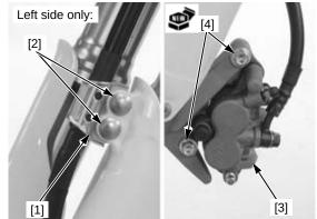
Inspect the wear rings [1] for wear or damage.
