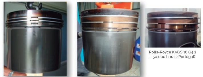
Rolls Royce Bergen K-G4 - 3000 horas (Teste Shell Global Solutions)
