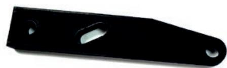
Figure 11.1. Resulting 3D-printed slider.
