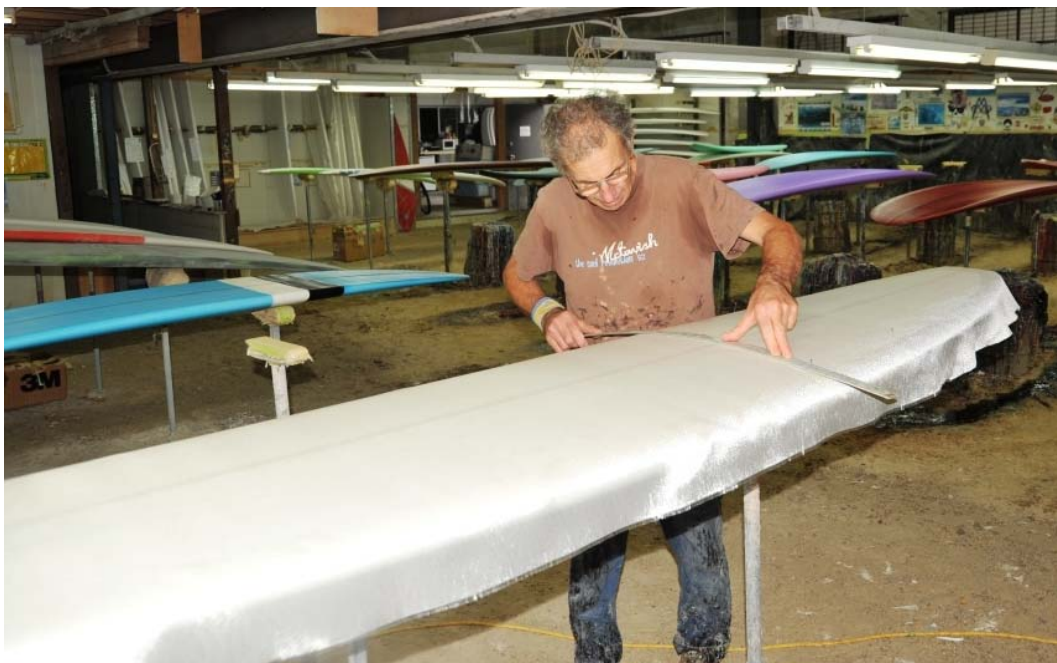
Figure 4.10: The 'lapping' of fibreglass cloth over the rails of the surfboard, before the 'hot' or fill coat of resin and catalyst is applied, Byron Bay. (source: Author)
