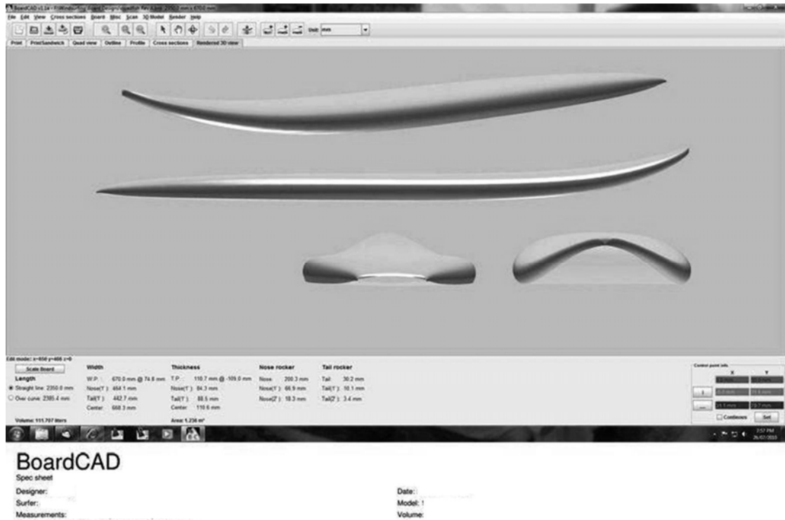
Figure 5.4: The computerised production system begins with programming a board design using the CAD system (source: Author)
