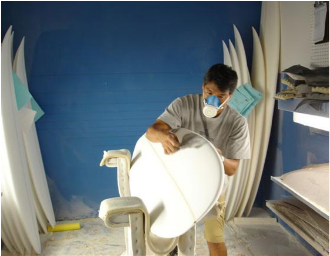
Figure 4.5: Eric hand-shaping in his shaping bay, Arakawa Surfboards workshop, O`ahu. (source: Author)
