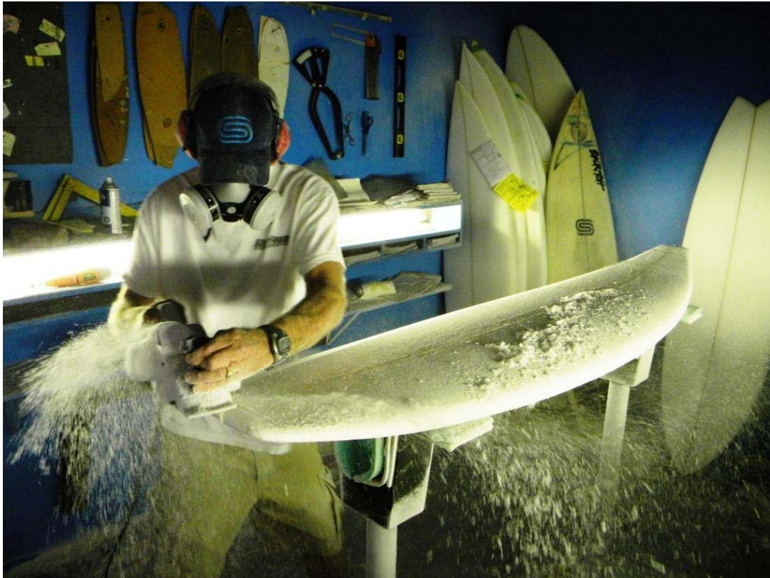
Figure 7.6: Greg from Sauritch Surfboards shaping a custom board using a respirator mask to ensure he doesn't inhale foam particles, southern California. (source: Author)
