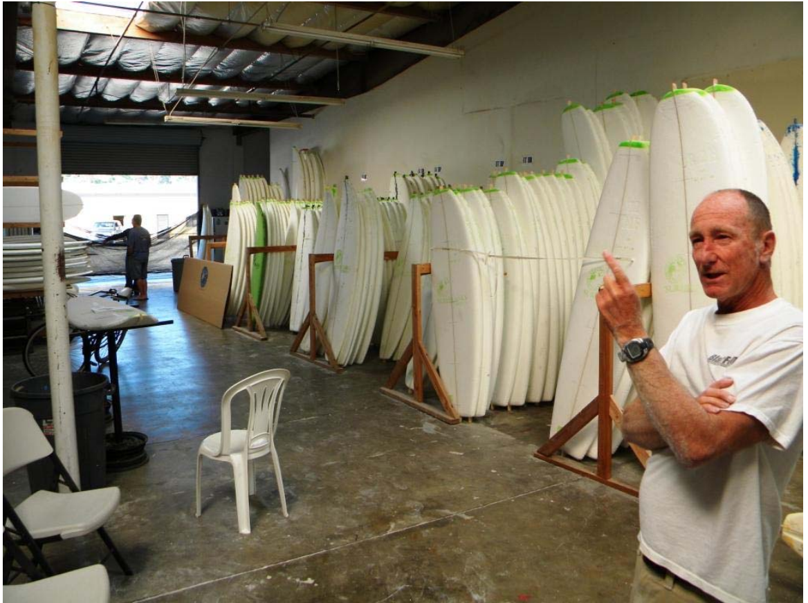
Figure 4.7: Greg from Sauritch Surfboards, southern California, showing hundreds of PU foam blanks. (source: Author)
