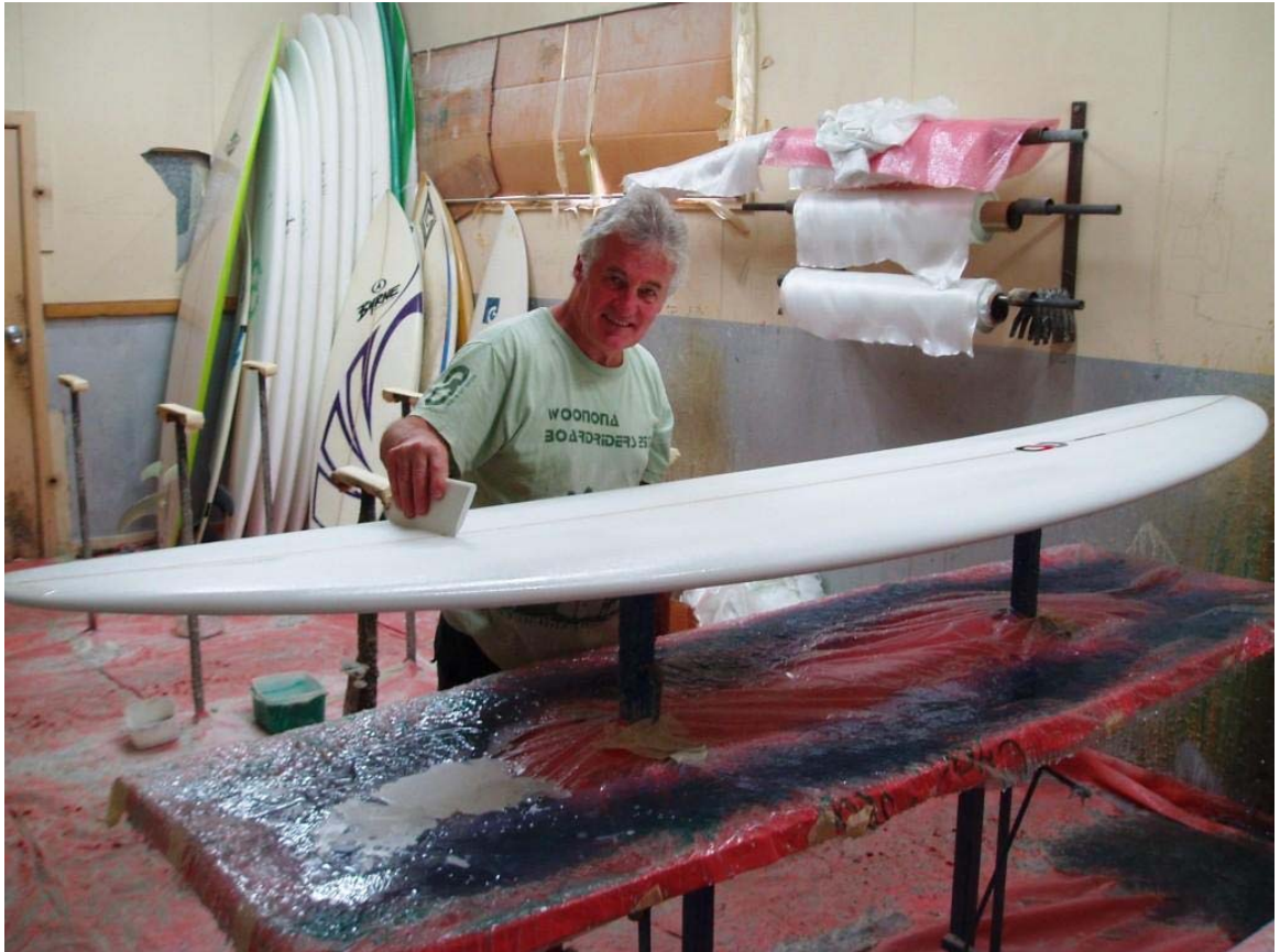
Figure 4.6: Mick glassing a new custom made longboard at the CSD workshop, Illawarra. (source: Author)
