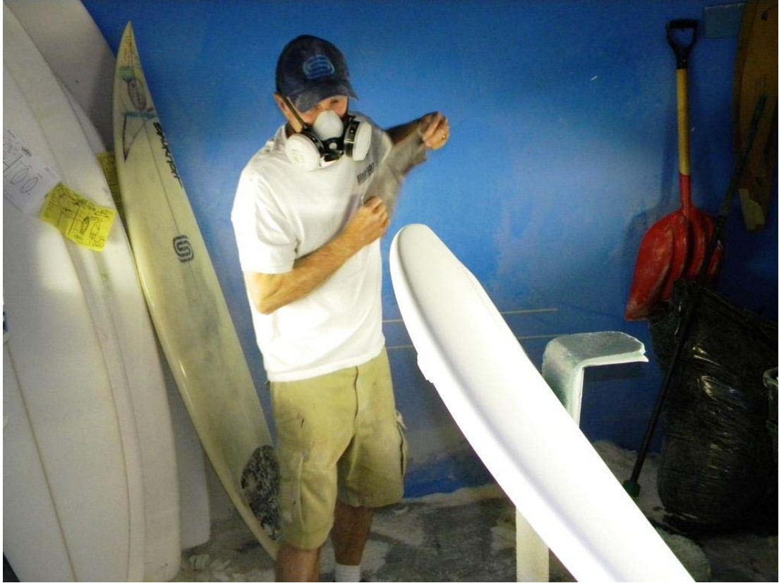
Figure 7.1: Greg using fly screen mesh to smooth over the rails of a custom board, southern California. (source: Author)
