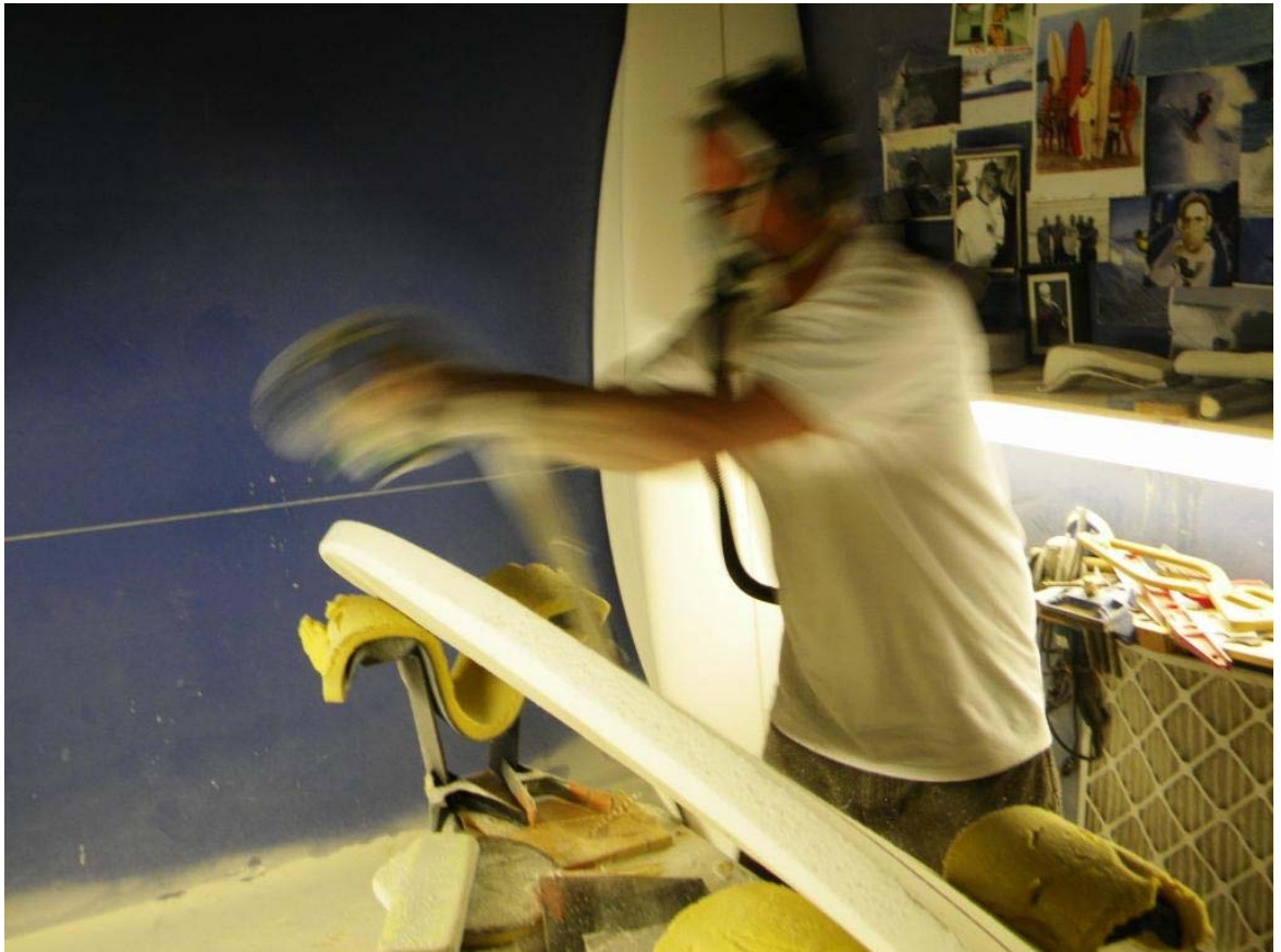
Figure 4.9: Tim Bessell in his shaping bay, using his Skil 100 planer to shape the rails to their correct thickness, southern California. (source: Author)
