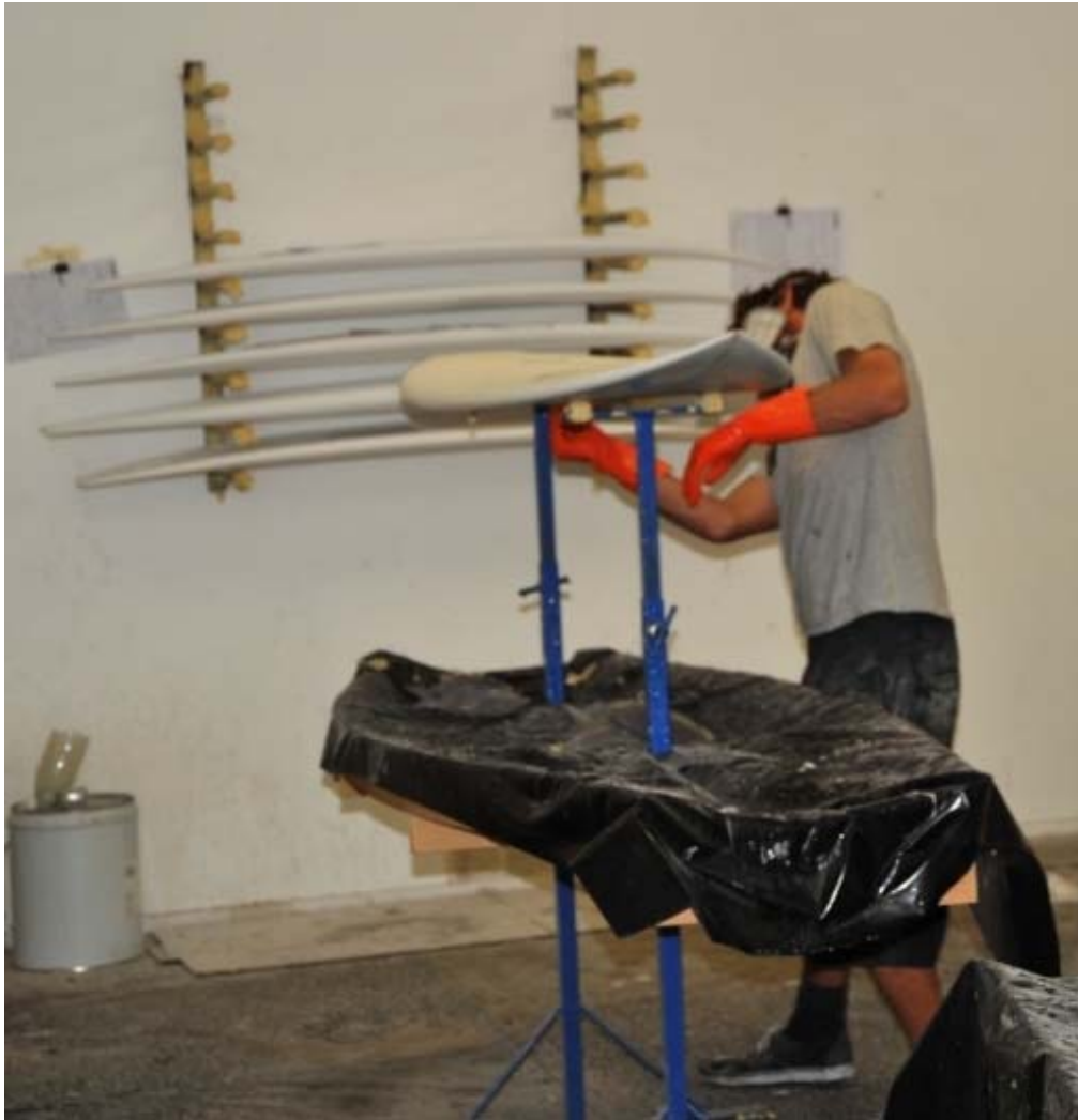
Figure 4.11: Applying the hot coat with a rubber squeegee, Gold Coast. (source: Author)
