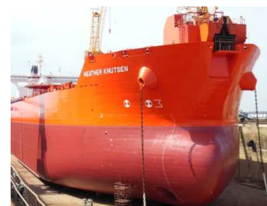
Tunnel thrusters one ahead + one aft Bow loading system
