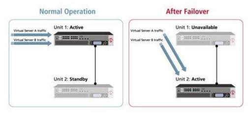
As you can see in the figure, unit 1 is in an active state, and unit 2 is in a standby state. With this configuration, failover causes the following to occur:
