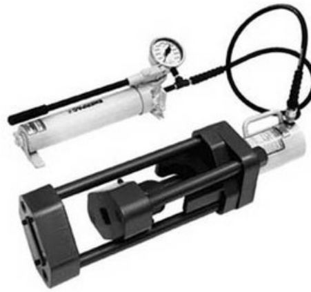
Figure 7-64.—Testing machine for making guided-bend tests. (Courtesy PCES Limited )
