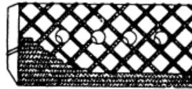
Figure 7-48.—Wearfacing bulldozer end bits.
