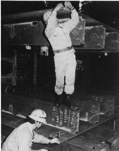
FIGURE 6-15: Specific A/C procedures apply to: A. Checking a measurement between panel and bracket edges in a sub-block. B. Checking a measurement between the edges of a panel and internal structure in a block. C. Checking alignment of a tank-top panel relative to a bottom-shell panel in a block. D. Monitoring bottom alignment between keel laying and launching. The distance measured is that from the bottom shell to a reference line marked on the vertical angle-iron which is fixed to the dock floor.
