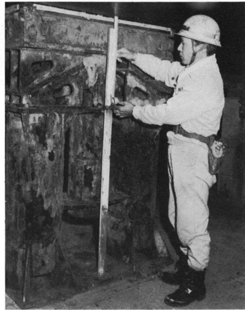
FIGURE 6-15: Specific A/C procedures apply to: A. Checking a measurement between panel and bracket edges in a sub-block. B. Checking a measurement between the edges of a panel and internal structure in a block. C. Checking alignment of a tank-top panel relative to a bottom-shell panel in a block. D. Monitoring bottom alignment between keel laying and launching. The distance measured is that from the bottom shell to a reference line marked on the vertical angle-iron which is fixed to the dock floor.
