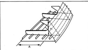
FIGURE 4-4: A and H are typical vital dimensions which A/C engineers require. Usually they are provided for in work instructions prepared by designers; loftsmen calculate their actual values.
