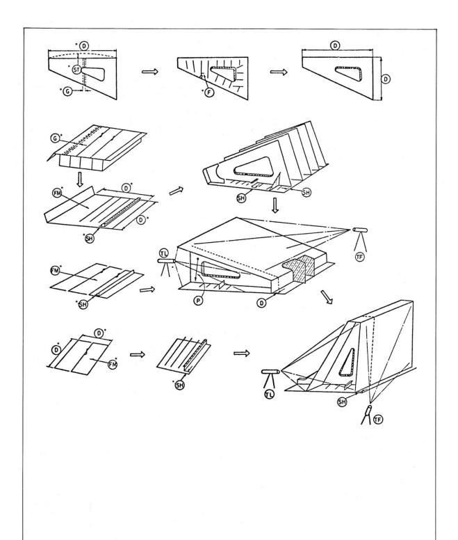
FIGURE 4-1: Dimensions and check methods that are typically the subject of check-sheet instructions for upper-wing tank parts in parallel midbody. See legend in Figure 4-2.
