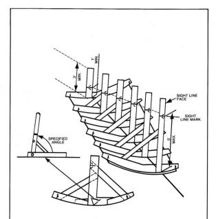
FIGURE 4-3: As shown, each template is set at a specified station and angle with its edge marks matching plate edges. Sight line marks, relative to a taut string, determine the accuracy of longitudinal curvature. Inclination of the sight line is an aspect of human engineering required as an A/C measure. A checker maintains an efficient, relaxed stance. Such techniques when repeated many times, significantly contribute to increased productivity.
