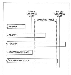
FIGURE 2-1: Accuracy exists in terms of a normally achieved range, i.e., a standard range. Learning how to work with ranges of variations is of great importanace, particularly for hull construction where shrinkages due to gas cutting, welding and line heating complicate sub-block assembly, block assembly and erection.
