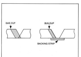
FIGURE 2-2: A/C focuses on minimizing rework on erection-joint gaps. The percentage of lineal measure of gas cutting and the percentage of lineal measure of back-strip welding, relative to the lineal measure of all erection gaps, are very effective productivity indicators.
