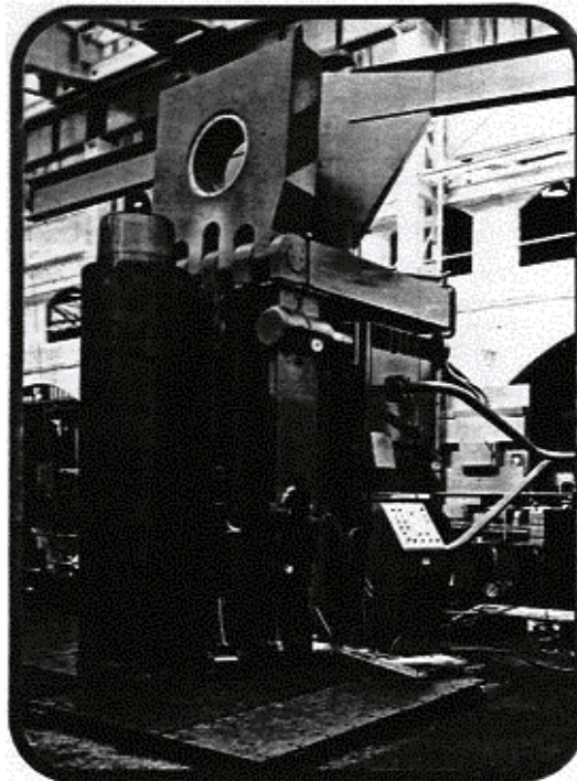
Shown Left: Hinged Slab (hydraulically operated) shown in the up position for removal of completed drums.
