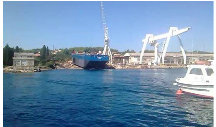
Figure 6. Recorded start of the launching closing to immersion
