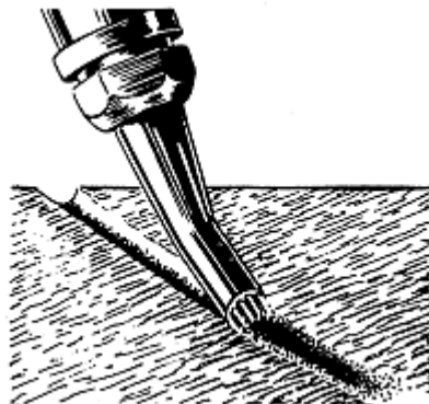
Figure 4-23. - Typical gouging operation using a low-velocity
