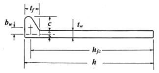
Fig. 21 Bulb profiles (DIN and JIS Standard)
