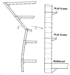
Fig. 18 **Reinforcement at knuckle**
