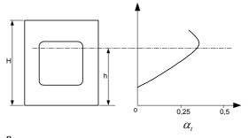
Fig. 8 Wash bulkhead coefficient
