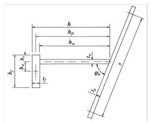
Fig. 20 Stiffener cross-section
