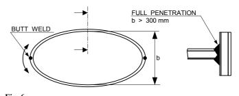
Fig. 6 Deck and bottom penetrations
