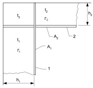
Fig. 12 Bracketless joint
