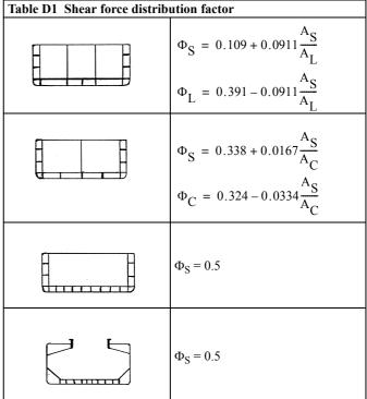
For these and other arrangements  $\Phi$  may be taken from a direct shear flow calculation.
