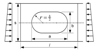
Fig. 2 Stiffening in direction of compressive stress
