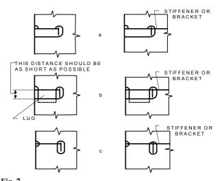
Fig. 7 End connections
