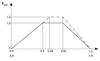
Fig. 4 Wave bending moment distribution
