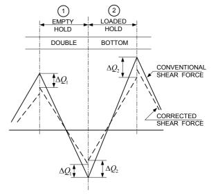
Fig. 8 Shear force correction
