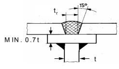
C: FILLED UP SLOT WELD
