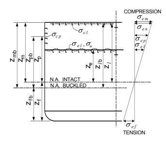
$\Delta M_{U} = additional moment above elastic buckling limit,$ to be taken as the smaller of: $<math display="block">\Delta M_{UP1} \Delta M_{UP2} \Delta M_{UP3} and \Delta M_{UF}$
