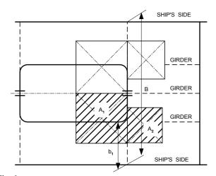
Fig. 6 Deck with transverse beams
