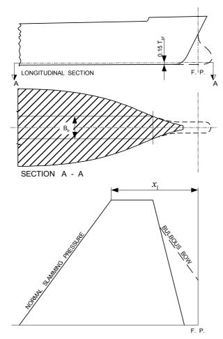
Fig. 2 **Design slamming pressure**
