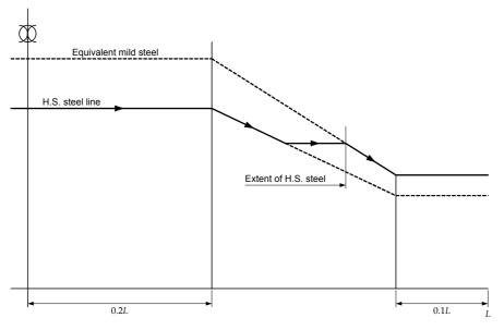
Fig. 7 Longitudinal extent of HS-steel
