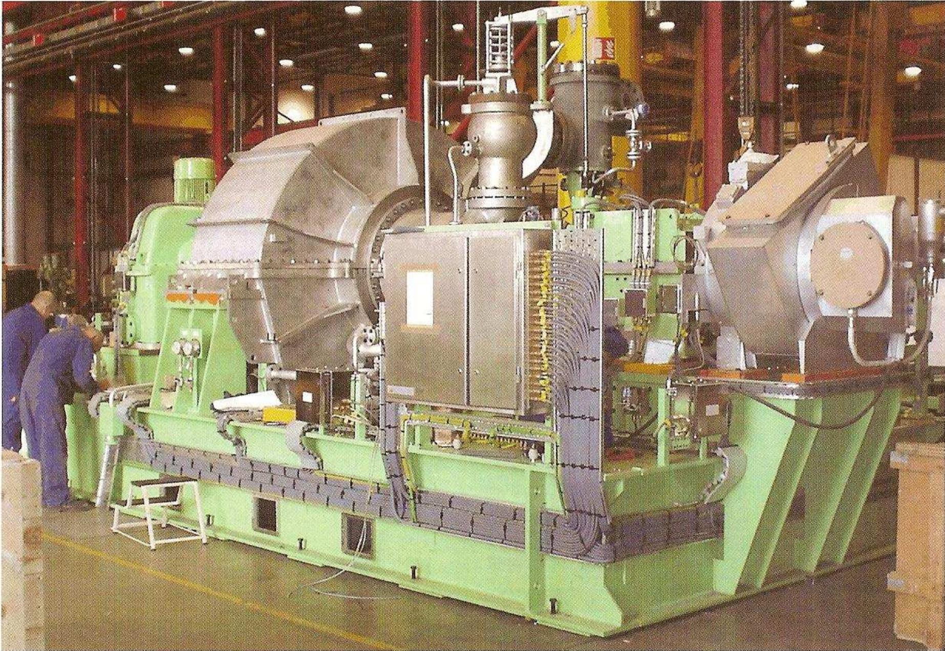
*The complete turbine generating set. The unit for an MAN B&W Diesel 12K98ME/MC engine measures only 10 m by 3.5 m.*
